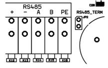
According to the RS485 specifications, the last device on the controller must be ending with a terminating resistor 120R. In the default configuration the jumper connector is not plugged. For each controller there is a separate termination resistor located behind the terminal block of the respective controller.
