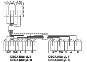
It is possible to connect up to 16 transmitters on each controller input, depending on their electrical distance from the controller.
