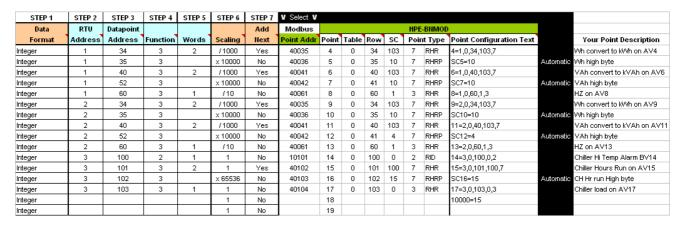
Once the information is properly entered in the tool the resultant point configuration data, in Column S, may be copied to Notepad for saving as a text file and download to the HPE-BNMOD.
