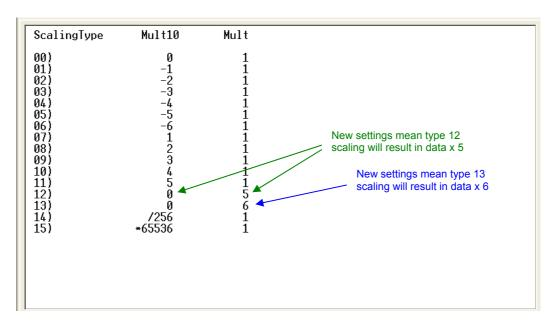
It follows that if type 8 Mult is changed to x7 (82=7) then the existing type 8 Mult10 (x100) when combined with the new Mult of 7 would result in object data multiplier of 700 when applied to a specific data object (data value x 100 x 7)
