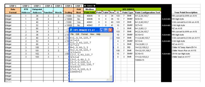
The last row of the download data, 10000=15, is a line count for a validity check as part of the download process. If manually entering the configuration text lines 10000=*n* should be ignored.
